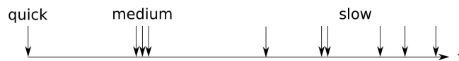
Figure 2 Waiting time of nodes in different states: A quick node creates a block instantly when seeing a new transaction. A medium node waits long enough to ensure not to compete with a quick node. A slow node waits long enough to ensure to compete neither with a quick nor a medium node. The figure represents a situation with one quick, three medium, and some slow nodes.
